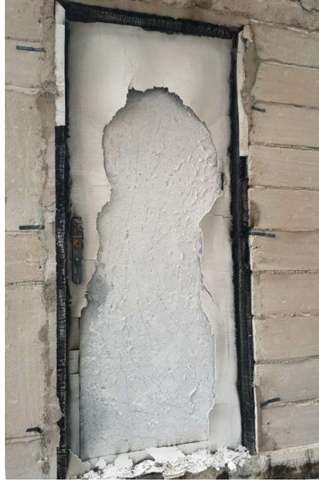
Photo No. 8 Exposed Side of Doorset B after 68 Minutes
