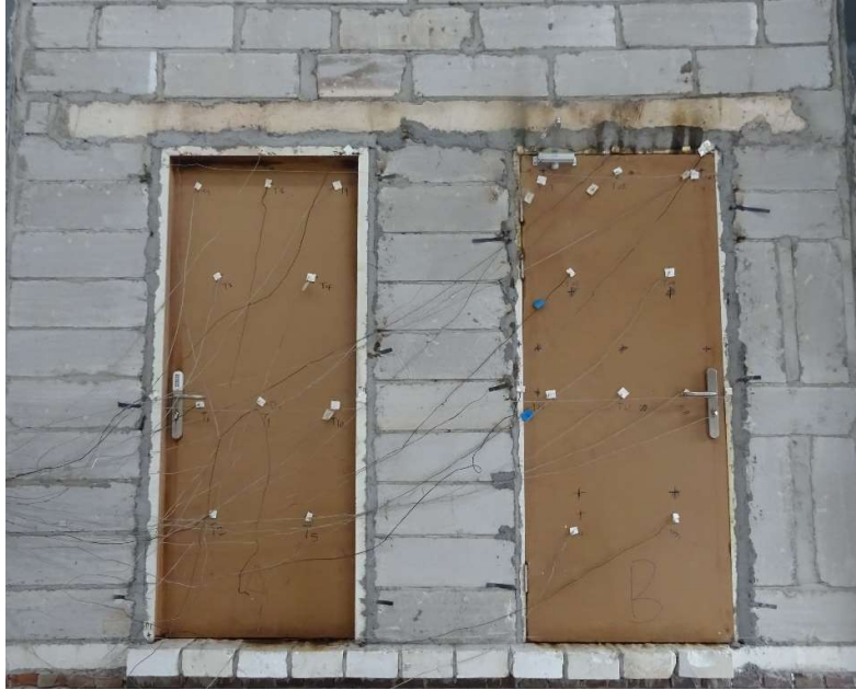
Photo No. 3 Unexposed Side after 10 Minutes
