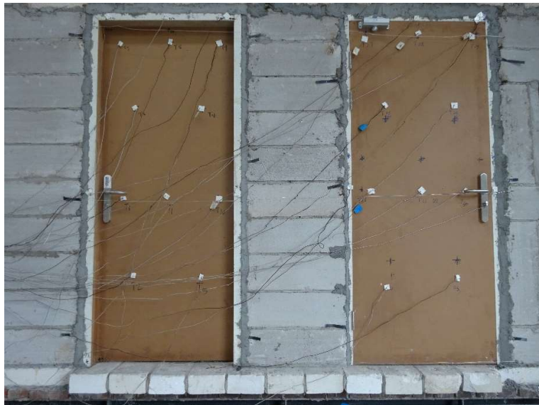
Photo No. 2 Unexposed Side Prior to the Fire Test
