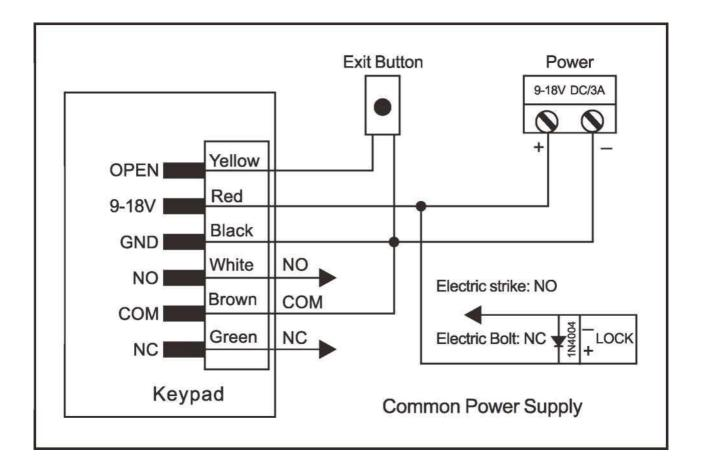
Attention: Install a 1N4004 or equivalent diode is needed when use a common power supply, or the keypad might be damaged. (1N4004 is included in the packing)
