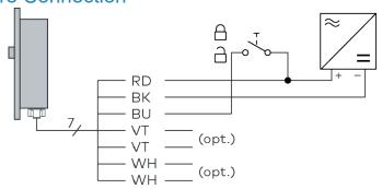
When in Fail Secure configuration, applying positive voltage to the control wire triggers the LC-MS1000P to unlock (active-low locking signal). In the event of a power cut, the LC-MS1000P will remain locked.
