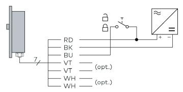
When in Fail Safe configuration, applying positive voltage to the control wire triggers the LC-MS1000P to lock (active-high locking signal). In the event of a power cut, the LC-MS1000P will unlock.
