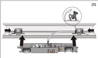
The screws must be removed before connect the mounting brackets to main case. Put the sensor into case and tighten the 2 mounting brackets to sensor.
