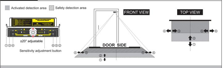
4) Every time you press the sensing range adjustment button, the detection range of the every corresponding edge (as shown in the figure) will move 1 level, total of 10 levels, until the sensor have beep beep sounds, means the detection range has been adjusted to limit, the limiting position of edge ③⑤ is center line.
